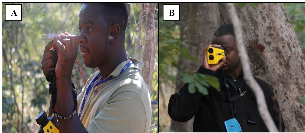
Figure 9: A- Bearing measurement using a handheld Compass. B- Distance measurement using a Rangefinder.
